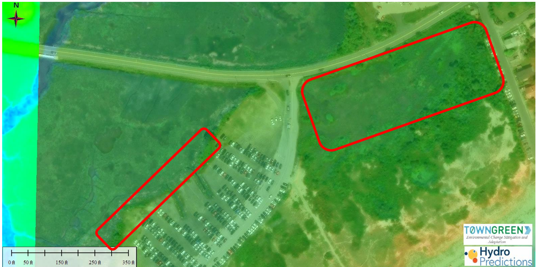
Figure 7. Good Harbor Beach Parking Lot Area - Restore degraded and filled saltmarsh adjacent to the Good Harbor Beach Parking lot east and west of the access road. Remove fill, restore natural tidal flow, and replace invasive species with natural vegetation. (GHBP-1 Latitude: 42.622312°; Longitude: -70.630980°; GHBP-2 Latitude: 42.621495°; Longitude: -70.633354°)
